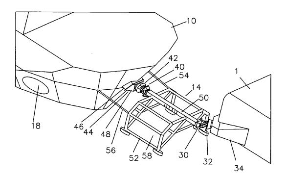
and service boat 10 to restrict rotational movement in the plane of the surface of the ocean, restricting the two vessels to a single degree of axial freedom relative to each other. When an extra degree of axial freedom is desired, tension can be released on cables or chains 54 and 56. Buoyancy material 58 is shown generally within the structure 52 to make the structure 52 positively buoyant.
